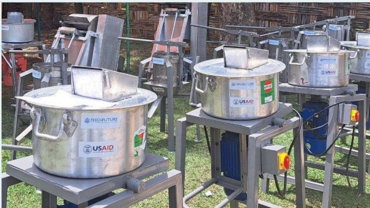
Enset corn miller machine, one of the new enset processing technologies
